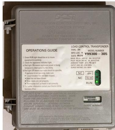
A green light on the LCT means the device is working and is not currently controlling your water heater or other device.
